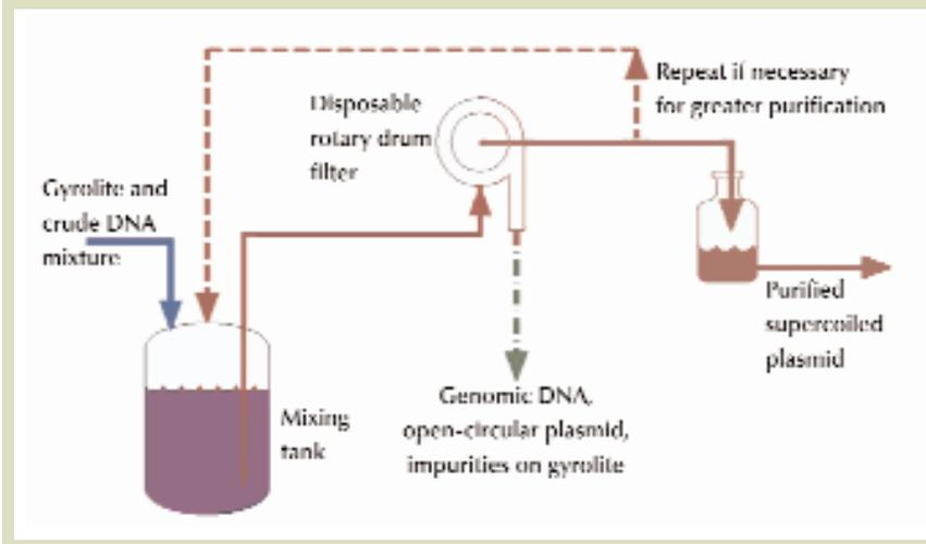
The resulting process creates an analog of a continuous chromatography system without the capital, labor, and resin expenses associated with column operation. As an added benefit, the equipment involved provides a method of processing material in an enclosed apparatus with a small footprint. And the disposability of the device reduces initial capital investment as well as the operating costs associated with equipment cleaning, validation, and such.
